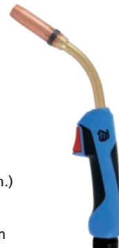
TBi 411 Classic Series 100% (10 min.) Mix: 450 A CO 2 : 500 A Ø 1.0-1.6 mm
