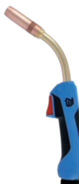
TBi 7W Top 2000 Series 100% (10 min.) Mix: 450 A CO 2 : 500 A Ø 1.0-1.6 mm
